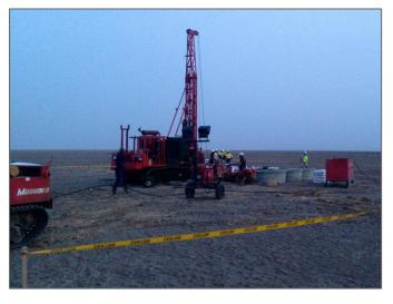
The drilling campaign completed during the quarter was used to collect resource data to support final pit designs and assess trafficability of the different materials within the resource to support mining fleet requirements and mine method.
