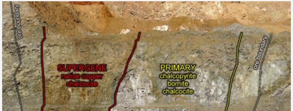
Top: Long-section of Las Minerale orebody, highlighting how native copper, supergene and primary ore will be accessed concurrently as the pit grows.
