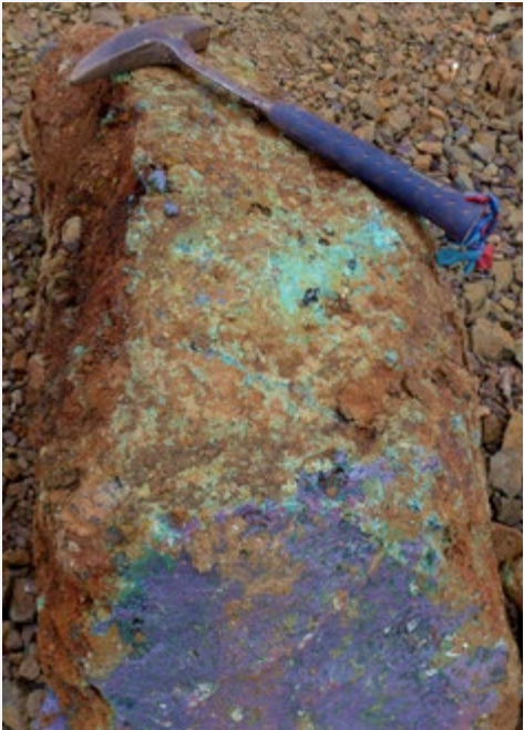
Executive Chairman Wayne McCrae admiring the rock-breaking of near solid cuprite and chalcocite boulders weighing up to 6 tonnes each. Right; detail of rock in hand showing near solid cuprite (cuprite contains 88.9% Cu) and native copper (native copper contains 99.8% Cu).
