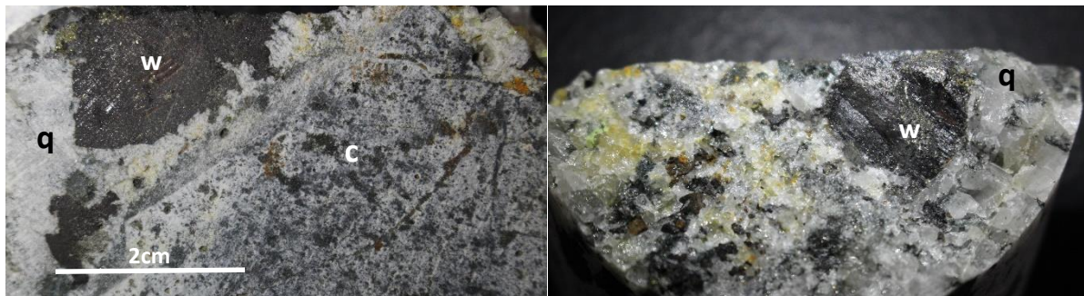
Figure 5: Wolframite at 59.3m within the upper hydrothermal breccia in CH-DDH012. LEFT: Cut core surface showing large wolframite crystal (w) in qtz matrix (q) adjacent to altered breccia clast (c); RIGHT: Broken core surface showing same wolframite crystal.
