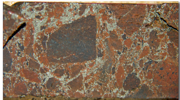
Fig 6. Shear hosted IOCG style high-sulphide zone intercepted by Talga at Kiskama.
