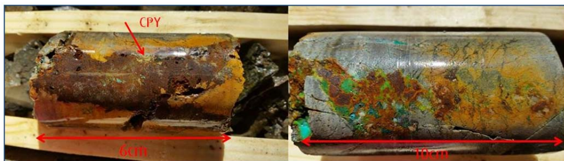
Figure 5: Copper mineralised drillcore from drillhole PAH05002. Approximate depth 136m.
