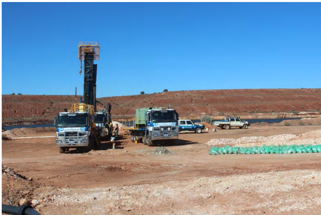
Figure 4: Diamond drilling at the Racetrack Prospect
