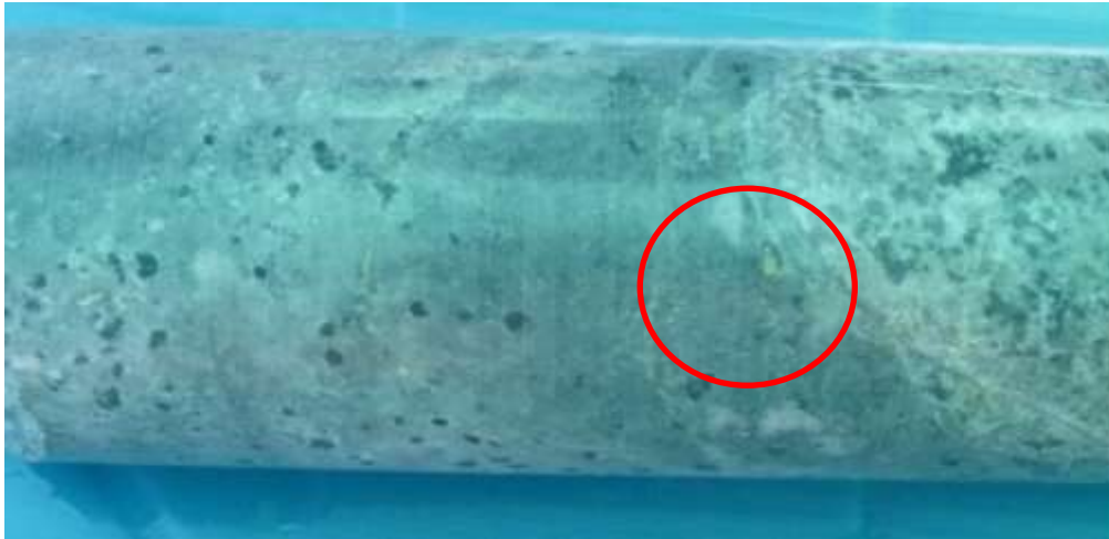
Figure 8 - (ALDD14006 drillhole depth 273.65m) Chalcopyrite in epidote-quartz veinlets (0.1cm wide), diorite intrusive, moderate potassic alteration (secondary biotite-orthoclase), moderate silicification.
