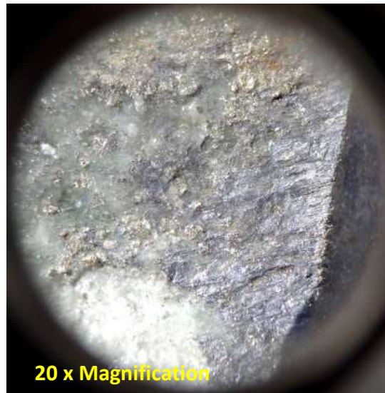
Figure 9 – (ALDD14007 Drill Depth 430.10m) Quartz-molybdenite-calcite veinlet, 2mm wide in andesitic tuff with strong phyllic alteration and 2% disseminated pyrite.
