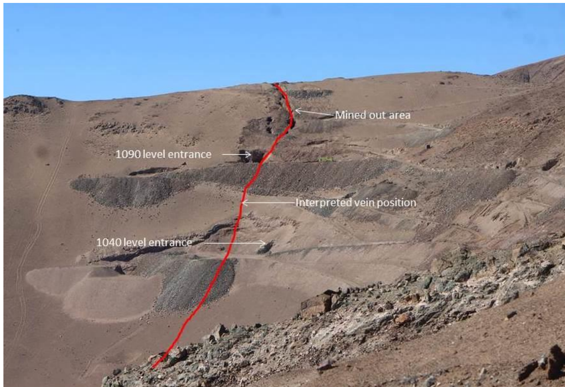
Figure 4 – San Sebastian mine and vein looking north. Note favorable topography for access, vertical distance between the 1040 Level and 1090 Level entrances is approximately 50m. It is planned that an additional level will be installed approximately 30m below the 1040 level entrance to access the vein.
