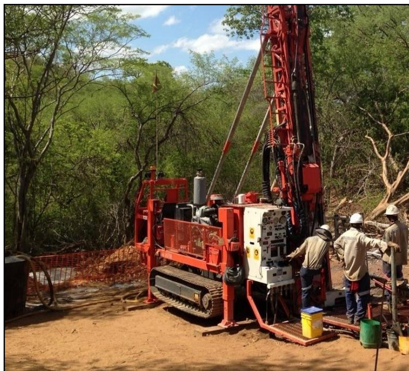
Figure 1. Two x DE710 Sandvik Drill rigs such as this one have been mobilised to the Montepuez Project.
