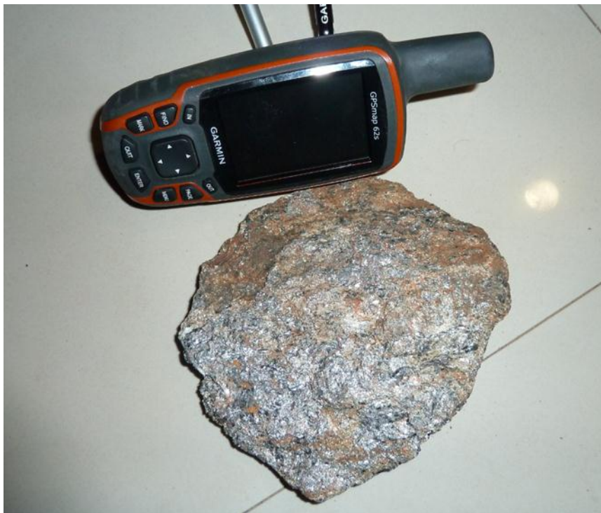
Figure 4: Grab sample from outcrop GBS02 displaying graphite mineralisation and large flake size.
