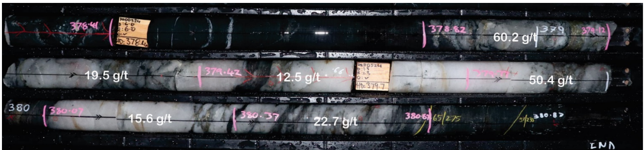
Figure 4: DRDD513 Milky quartz veining with narrow zones of smoky grey quartz. Equal amounts of pyrrhotite and chalcopyrite fracture fill. 20+ flecks of visible gold. Interval assayed 1.9m @ 58.0 g/t gold.
