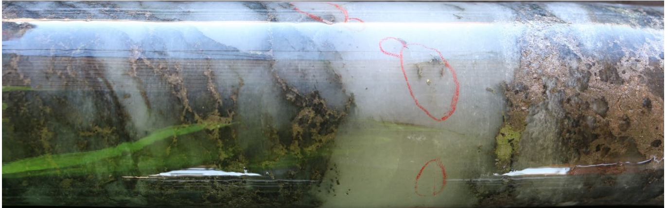
Figure 2: DRDD521 444.6m-445.5m. Smokey grey quartz vein with moderate pyrrhotite and chalcopyrite fracture fill in addition to trace arsenopyrite. Vein has 20+ flecks of visible gold, largely associated with a hairline fracture through the full thickness of the vein. Assays pending.
