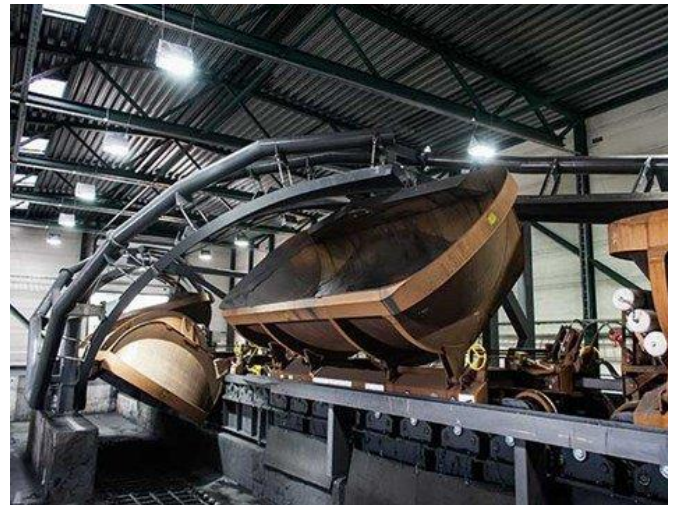
Conceptual example of ‘Helix Dumper’ in operation. Image is not a representation of actual infrastructure at the Port of Esperance. (Image reproduced with permission from Kiruna Wagon & RCR MT)
