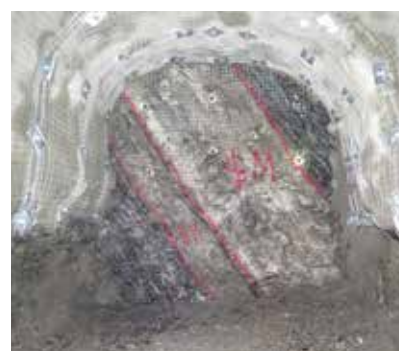
TBA 460 ore drive (4.5m W x 4.5m H) with a face grade of 5.7% Ni
