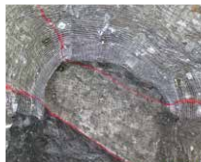
SBA 737 ore drive (3.5m W x 3.5m H) with a face grade of 6.2% Ni
