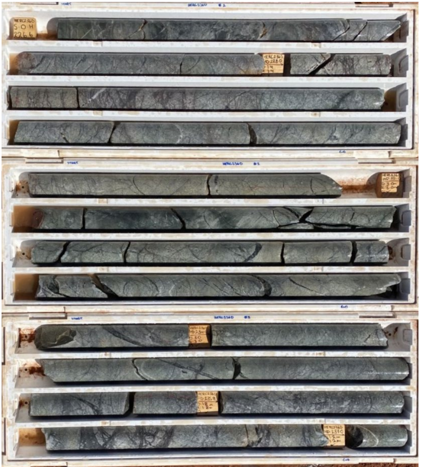
Figure 5 Falcon HERC236D – Photograph of strong sulphide rich alteration and brecciation from 226.6m to 237.1m (results pending).
