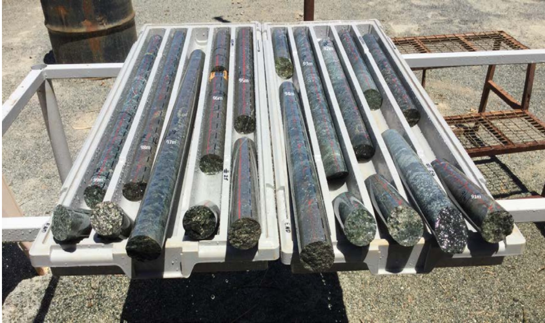
Figure 3: Nickel-copper sulphide mineralisation in drill hole ANDD0001: 90.4m – 99.2m
