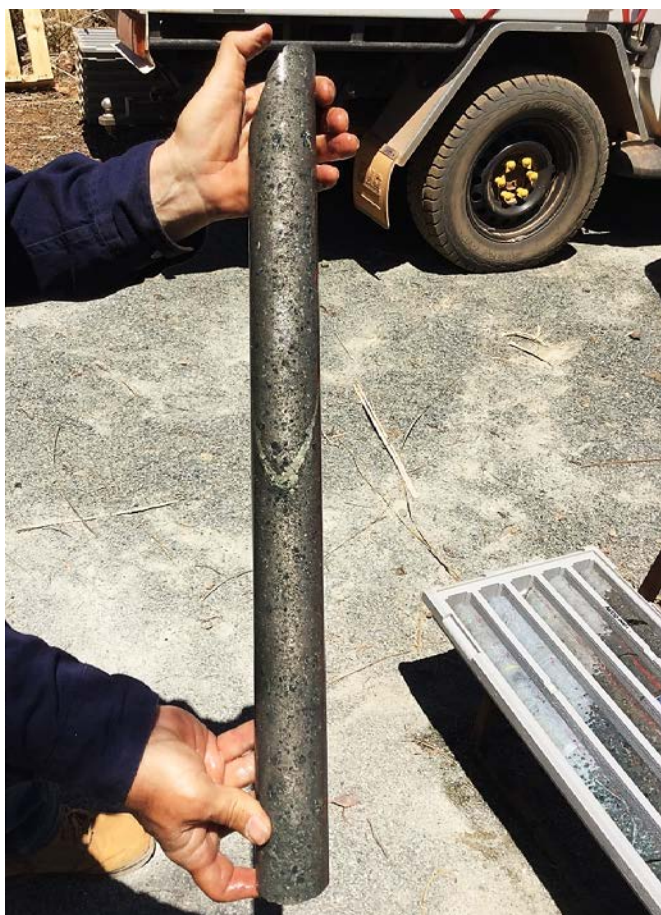
Figure 1: Massive nickel-copper sulphides from ANDD0001: 94.6m - 95.5m downhole
