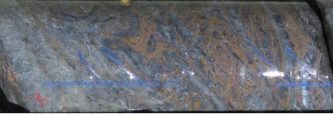
OFDD003: sheared quartz-sphalerite (271.65 - 271.8m)
