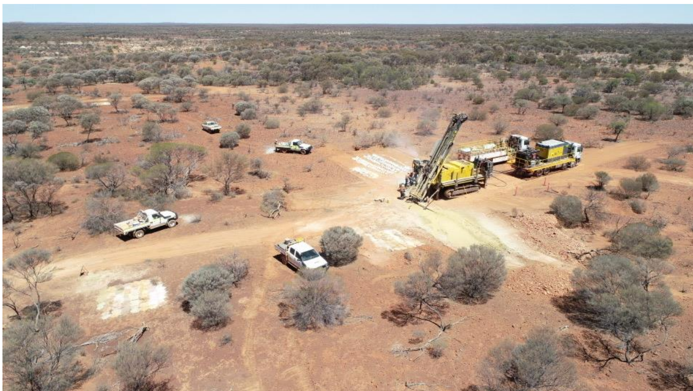
Figure 1. Reverse Circulation Drilling underway at Target 1
