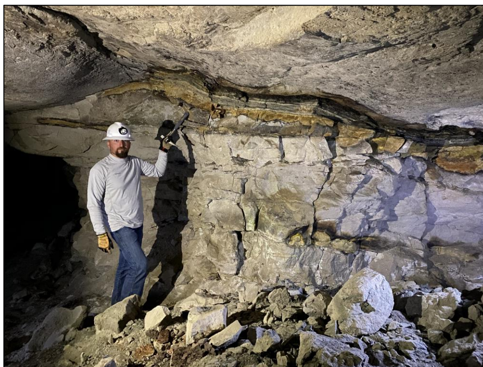
Figure 2: Photos of visible uranium and vanadium mineralisation associated with high-carbon stratification and localized remobilization within historical underground workings of the Yellow Cat project.
