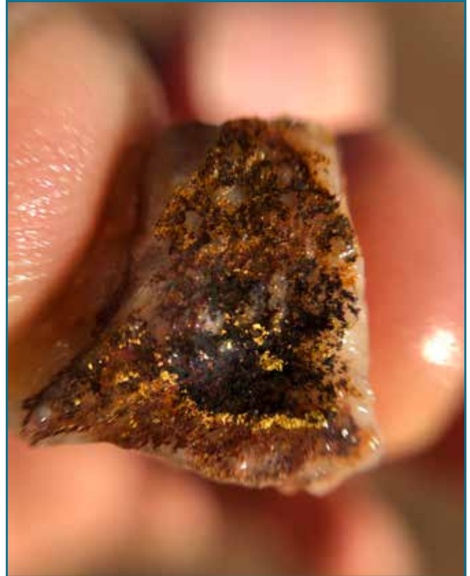
Visible gold in RC quartz chips from the Starlight lode at Break of Day, 20MORC068, 6-7m, 1m @ 2,518.8g/t Au within 14m @ 191.1g/t Au from 4m
