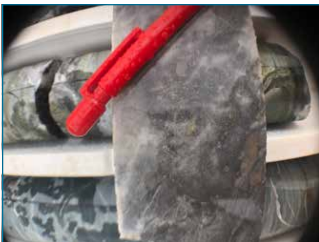
Visible gold in core from the White Light lode at Break of Day, 20MODD007, 100.2m, 0.75m @ 203.3g/t Au
