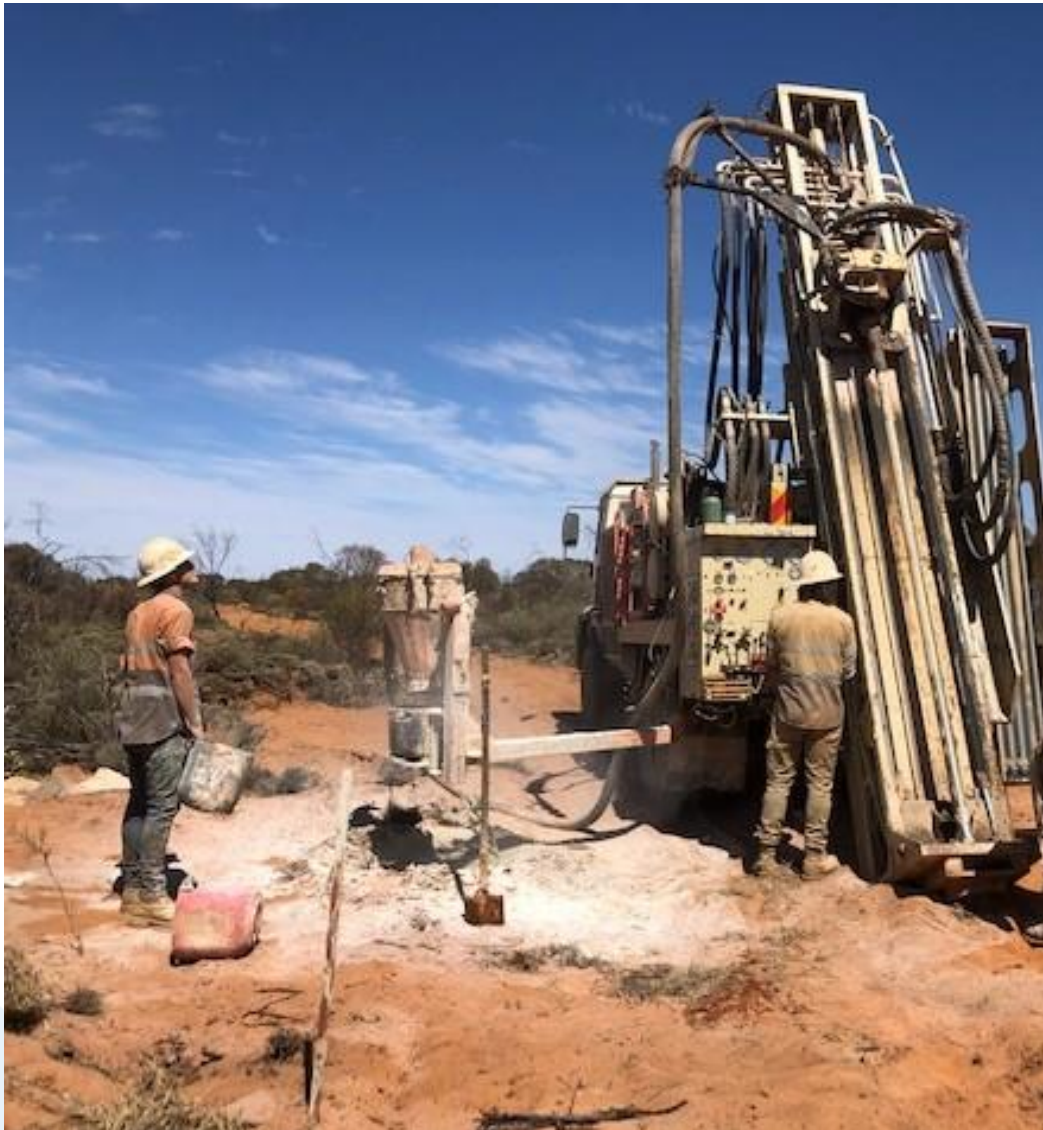
Figure 5. Aircore drilling of regional targets at Rox's regional tenements (100%) at the Youanmi Gold Project
