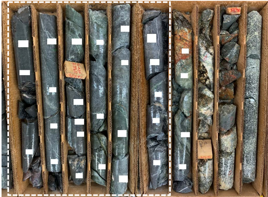
Figure 4 - WT-20-05 – Fine grained chalcocite rich mineralisation observed within skarn over ~8.4m
