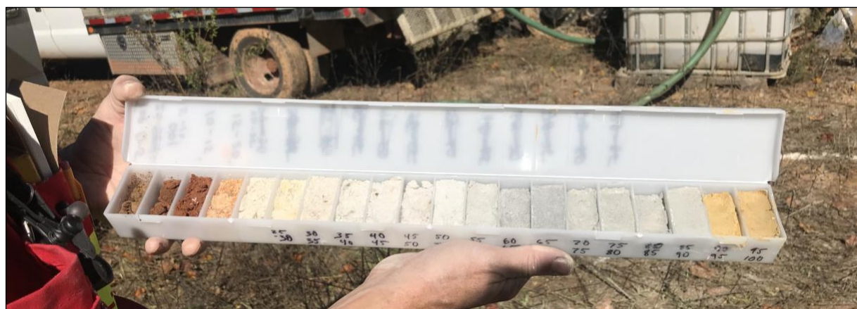
Figure 1: First hole chip box showing 1.5 metre (5 foot) intervals of drilling at the Titan Project
