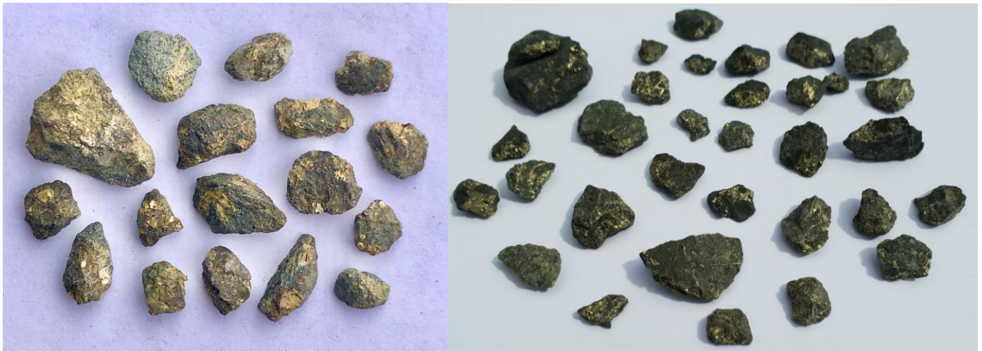
Figure 1. Disseminated chalcopyrite and pentlandite in drill chips from ultramafic rocks at Platinum Springs East (left: PSIPT019 42-44m) and Plat Central (right: PSIPT030 from 62-63m at Plat Central). The chips are up to 2 cm in dimension.
