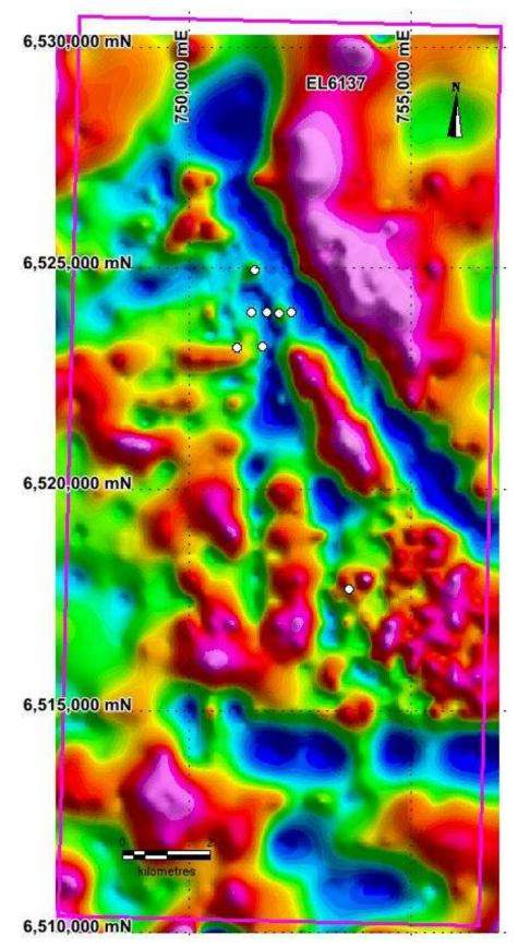
Figure 2: EL 6137. Residual gravity image showing locations of proposed drill holes (white dots). Grid GDA 94 Z53.
