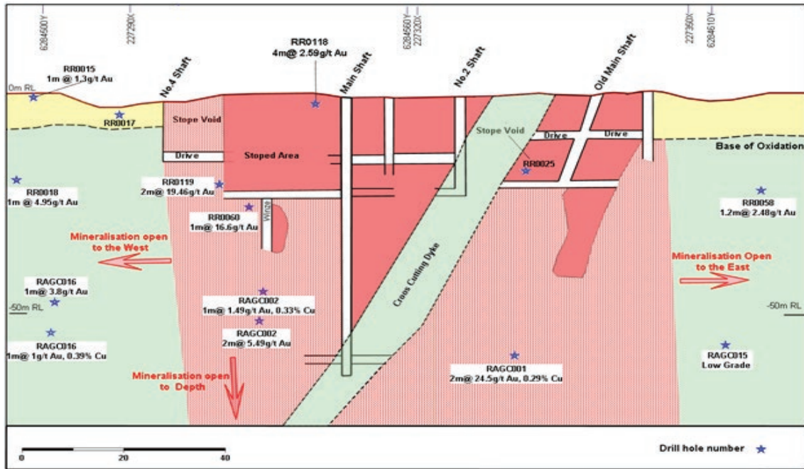
Figure 3. A long-section of the Maori Queen Mine showing the old mine working and drill hole intersections
