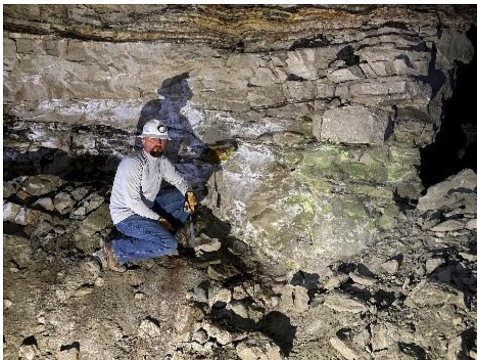
Figure 6: Photo showing visible uranium and vanadium mineralisation in the workings at Yellow Cat.
