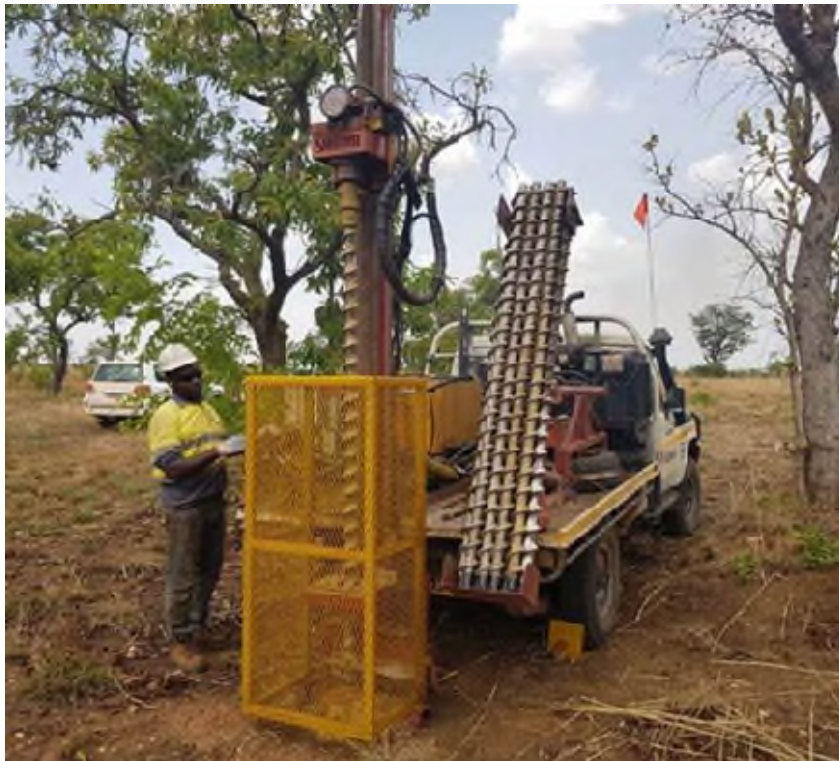
Vehicle mounted auger drilling unit
