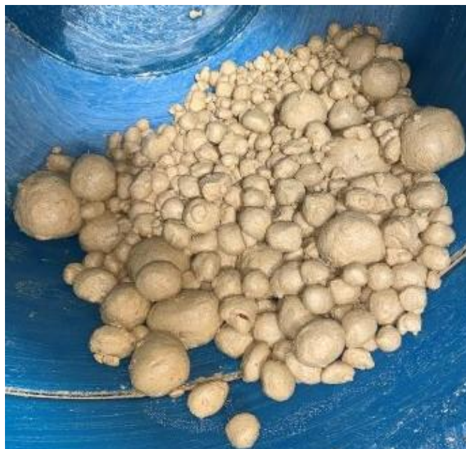
Figure 2 - Agglomerated co-mingled tailings and waste rock for disposal to waste rock storage
