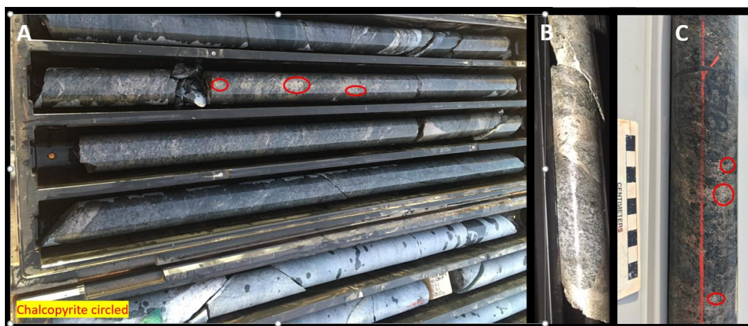
Figure 1 | Diamond drill core from McKenzie Springs A) FNDD002 semi-massive to foliation disseminated sulphides from 276m B) FNDD002 semi-massive sulphides C) FNDD002 breccia textured sulphide (pyrrhotite-pyrite-chalcopyrite) at 278m
