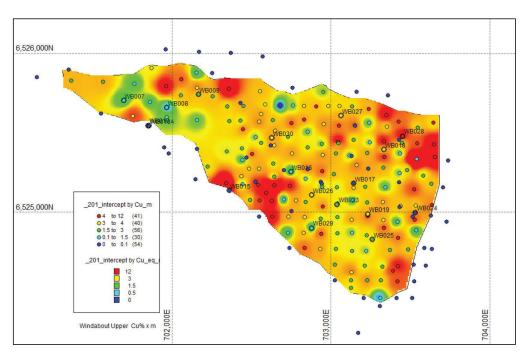
Figure 2-8: Windabout modelled mineralisation in plan view (upper horizon)
