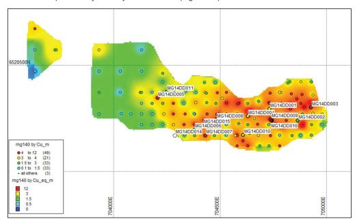
Figure 2-7: MG14 modelled mineralisation in plan view
