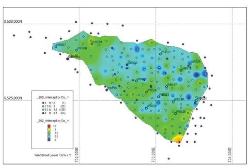
Figure 2-9: Windabout modelled mineralisation in plan view (lower horizon)
