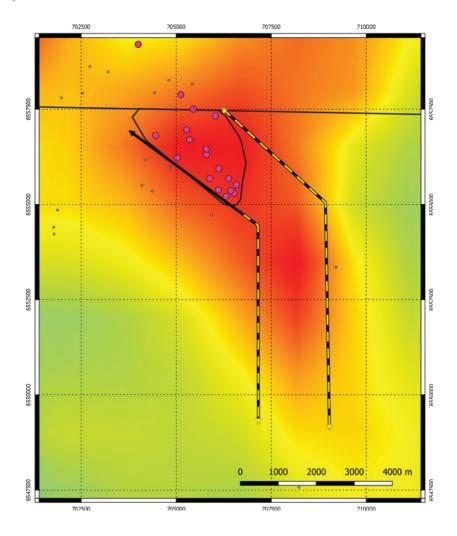
**DIAGRAM 6:** Magnetotelluric depth slice at approximately 390m deep showing coincidence with historical mineralised drilling at Emmie Bluff.
