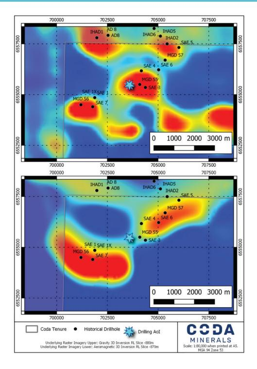
**DIAGRAM 4:** Elaine proposed drilling over gravity (above) and magnetics (below). Drill collars have been filtered to remove all holes which did not intersect basement.
