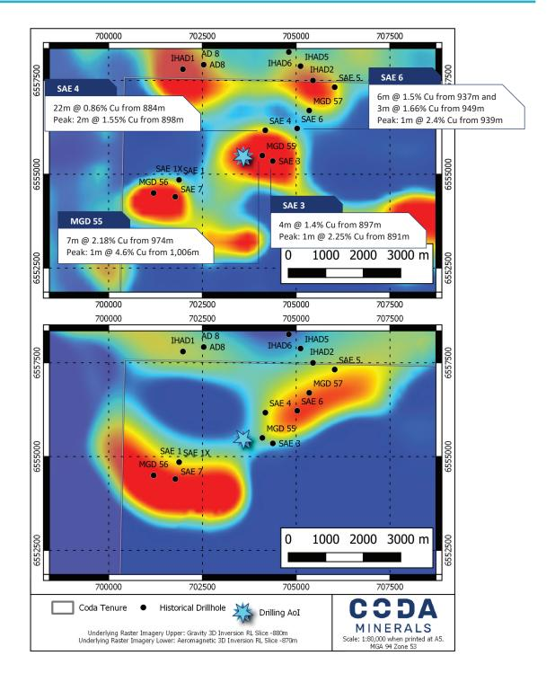
**DIAGRAM 3:** Emmie Bluff Deeps proposed drilling over gravity (above) and magnetics (below). Drill collars have been filtered to remove all holes which did not intersect basement.
