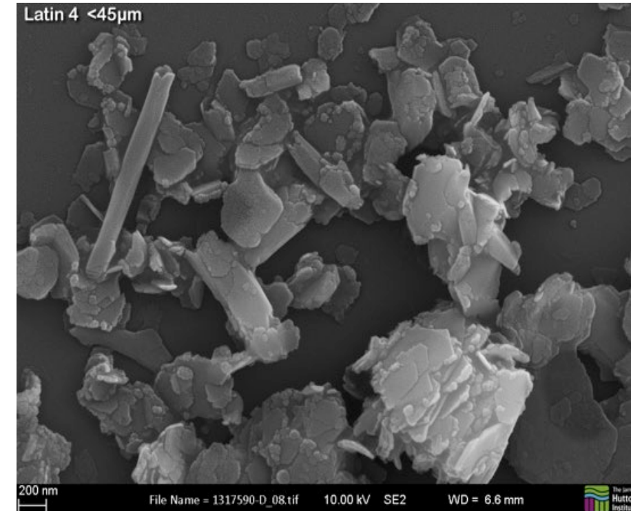
SEM image of <45 micron fractions showing halloysite tubes and kaolinite plates from location 4 (NB4)
