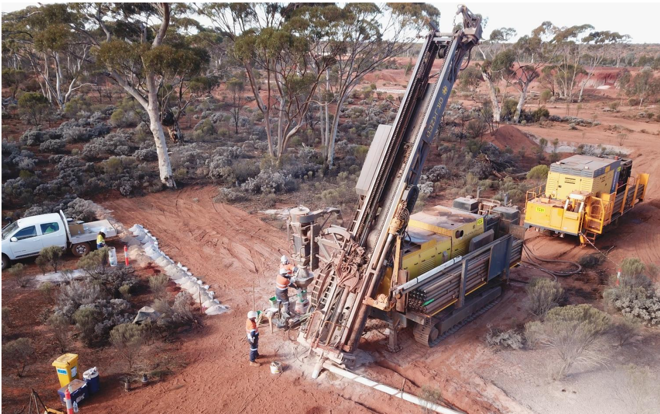
Image 4 – RC drill rig at Mandilla East
