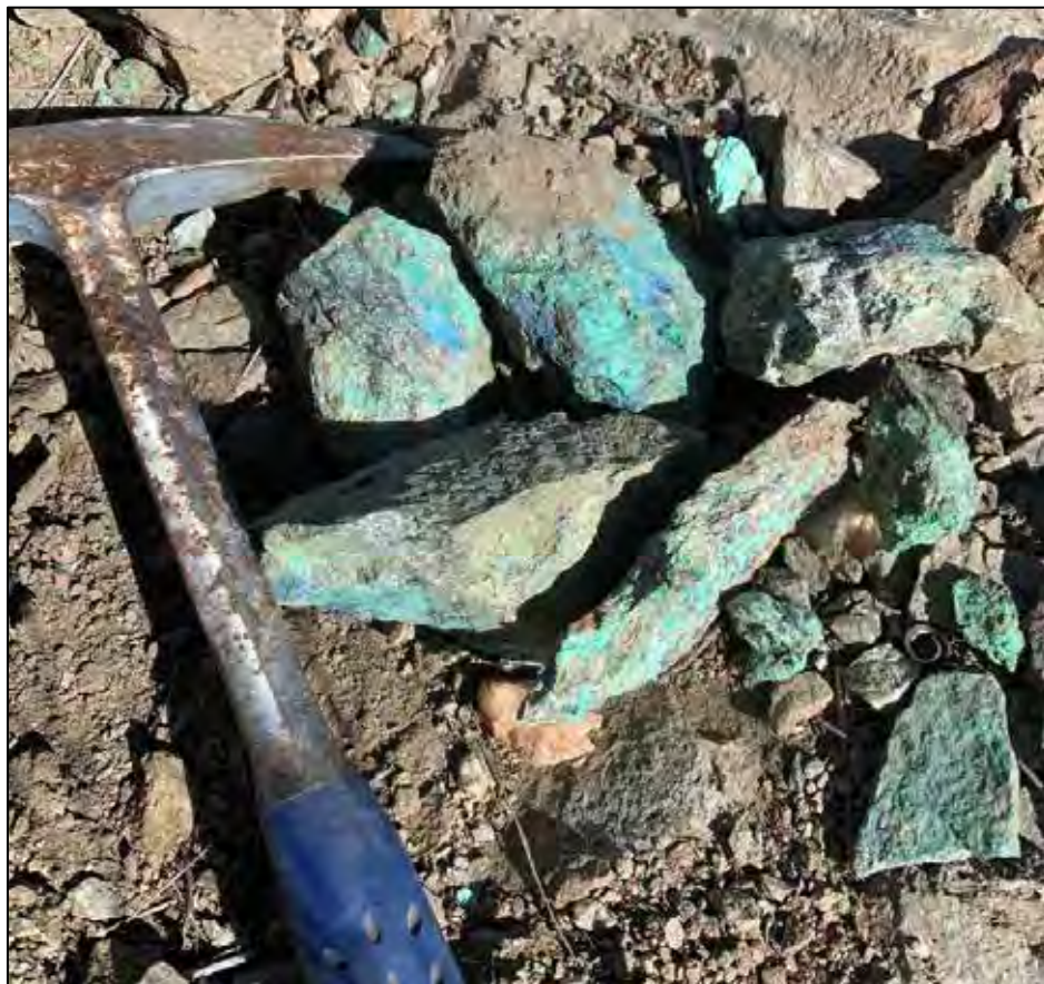
Photo 7 - High-grade waste from dump material at OREX target assaying 9.15% Cu, 192 g/t Ag and 0.15 g/t Au. The sample was collected next to a small adit mined along a copper-bearing shear within the Leatherwood intrusive.
