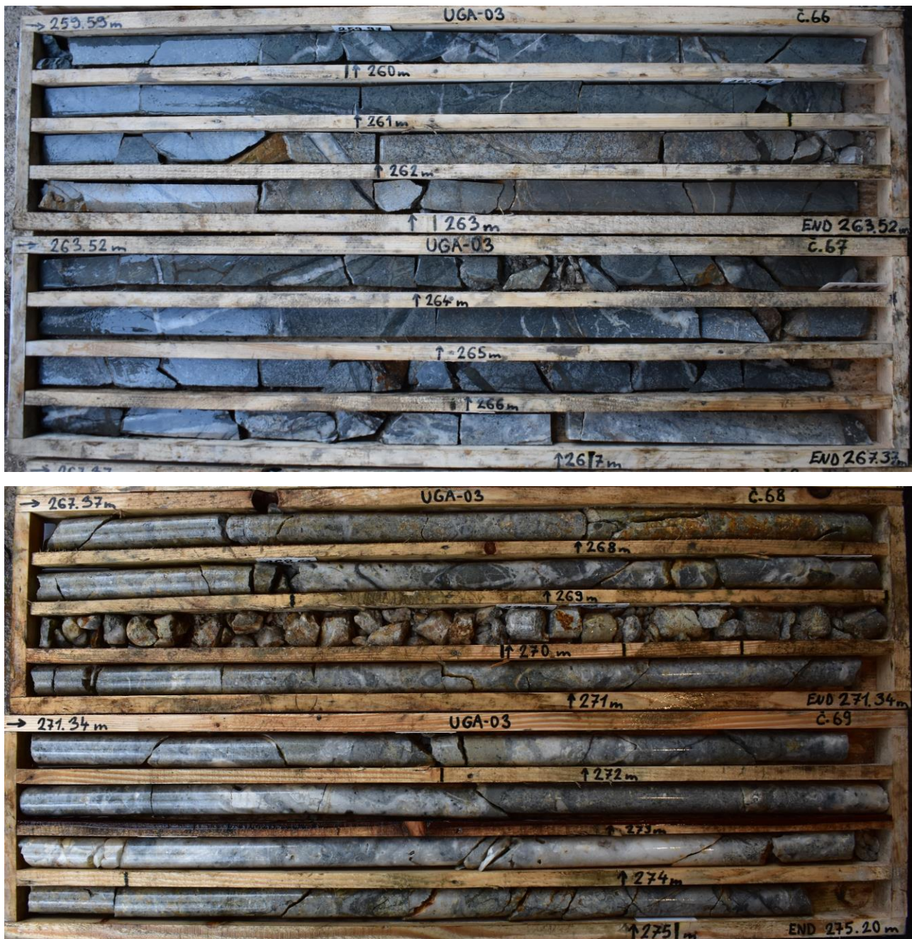
Figure 1: Drill core photos from UGA-03 showing an example of rocks within the Schramen Vein zone, which is a quartz filled vein/stockwork/breccia zone, variably rich in fine grained sulphides (mainly pyrite) and hosted within strongly leached and argillic altered andesite host rock
