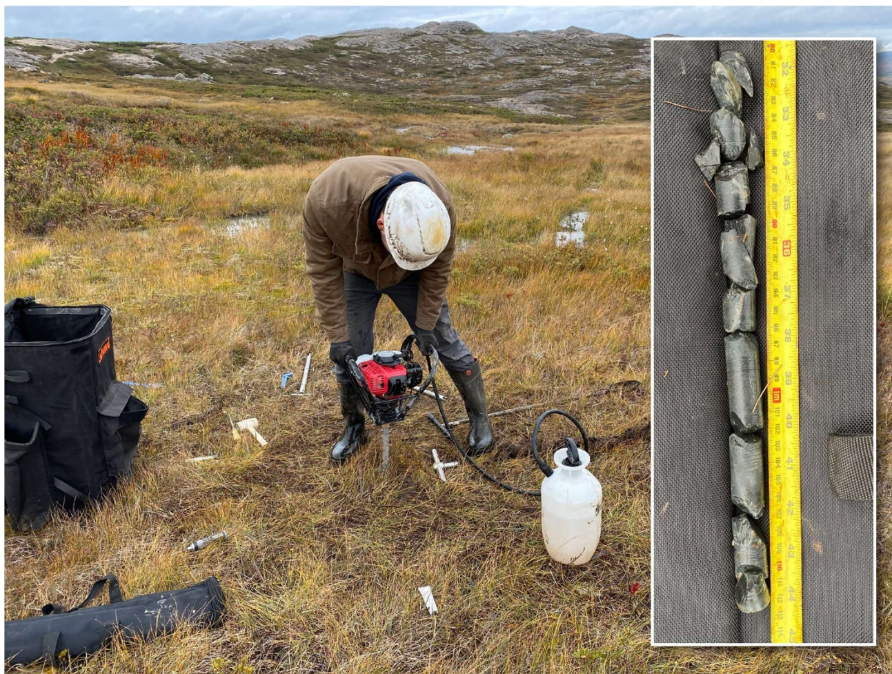
Figure 6: Person-portable backpack drill unit in operation, collecting soil, till and short in-situ basement drill core samples for multi-element geochemistry and spectral data analysis.
