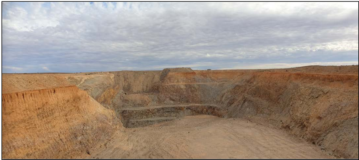
Figure 19: Existing shallow Vertigo Pit facing south west, mineralisation extends gently downward from the south eastern (left) side of the pit
