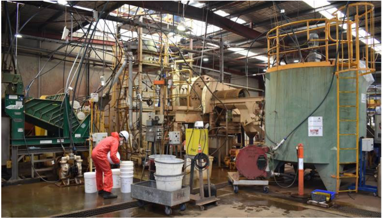
Figure 2: Comminution section of the beneficiation pilot plant at ALS Metallurgy, Perth, showing, SAG mill, vibrating screens and flotation feed tank on the right
