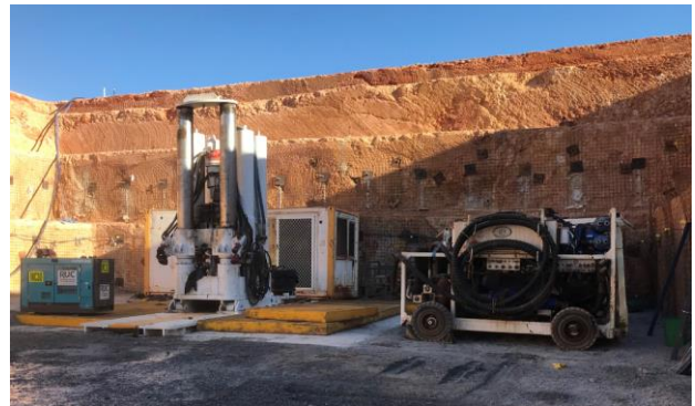
Raise bore machine set-up in box-cut
