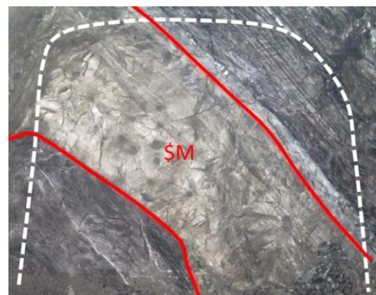
445 ore drive (4.5m W x 4.5m H) with a face grade of 5.5% Ni
