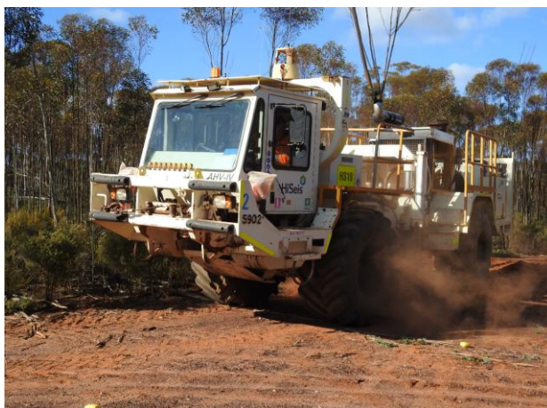
Vibroseis Truck in Action at Spotted Quoll
