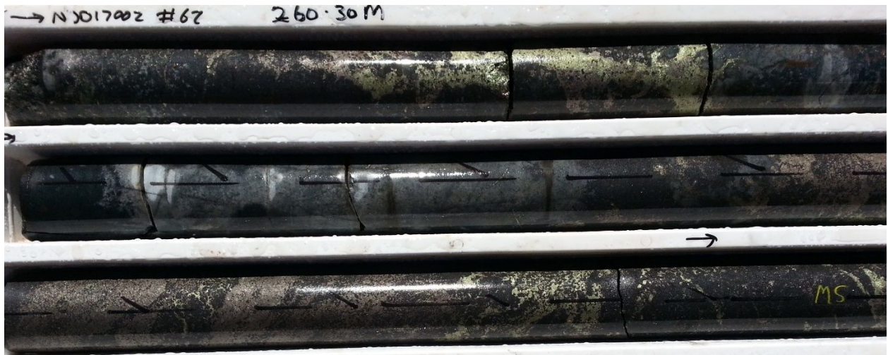
Image 1 / Stark stringer sulphides (chalcopyrite/pyrrhotite/pyrite) 260.3m to 263.1m in NDD17002
