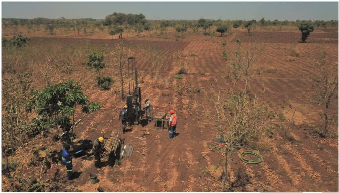
Figure 9: Drone photograph of the push-tube core rig in action at Kasiya.
