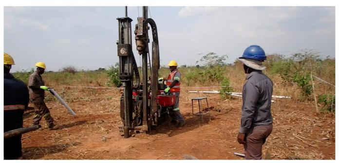
Figure 3. Push-tube core drilling at Kasiya.
