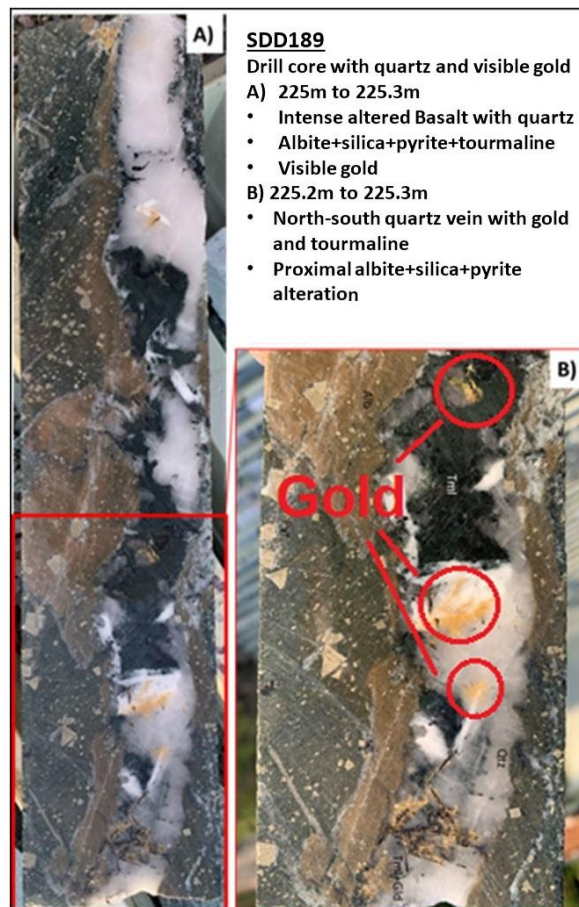
Figure 3 – SDD189 – High grade intercept of 1m at 1176.99 g/t Au from 225m with strong alteration and multiple occurrences of visible gold.
