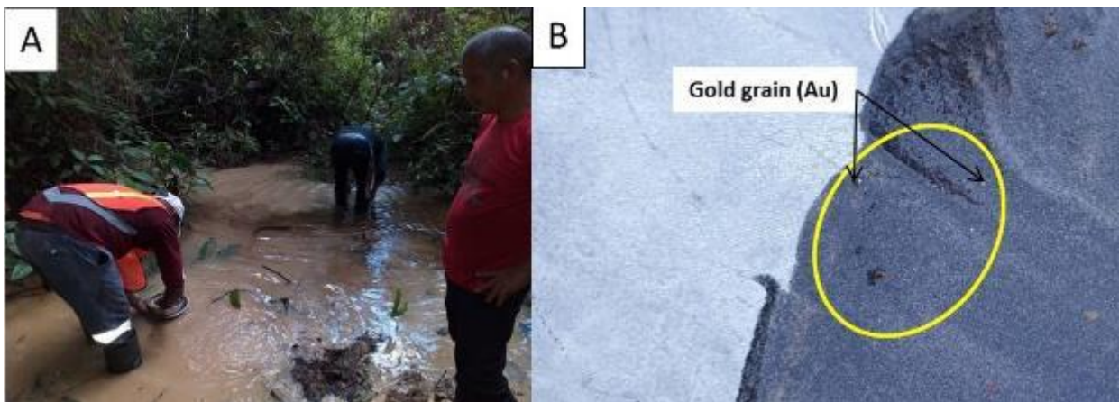
Figure 7 - (A) Panning and sieving of samples (B) Visible gold grains in pan from point BSS002 (see map below)
