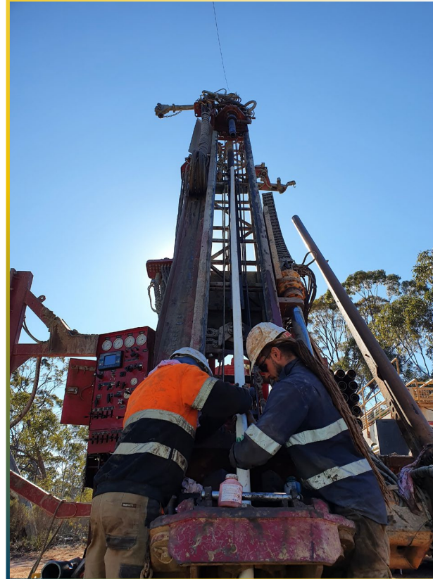
After completing the RC drill hole offside from Red Rock Drilling carefully lower PVC pipe down the hole enabling down-hole geophysical surveys to be completed at a later date (October 2020)
