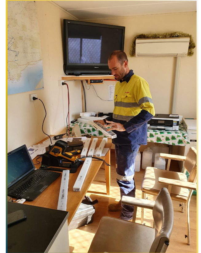
Geologist Tony Pfaff completing XRF analysis of RC drill chips at the Forrestania camp (October 2020)
