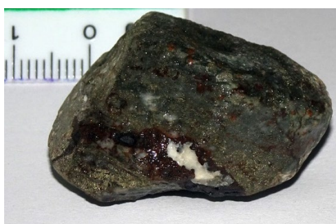
Figure 5: Aircore sample from hole JSA20_175 at 91-92 metres (end of hole) showing phyllic (Quartz-Sericite-Pyrite) alteration and Quartz-Hematite veining with pyritic vein selvage.
