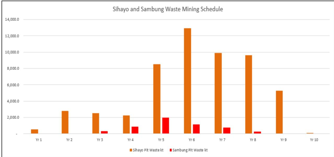
Figure 6-17. Sihayo and Sambung Waste Movement Schedule
