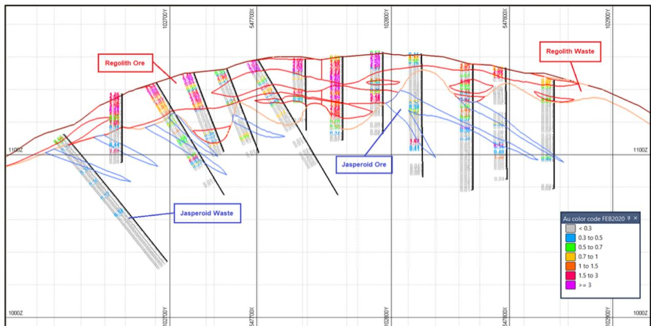
Figure 4-1. Figure 56 Sectional view of infill and ore grade population strings
