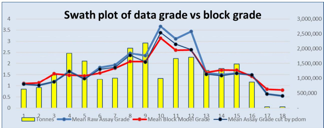
Figure 4-4. Sihayo Sectional Swath Plot (Figure 67)
