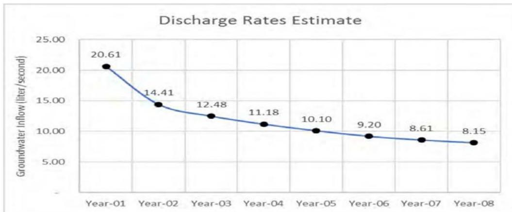
Figure 6-20 Groundwater inflow rates of Sihayo pit
