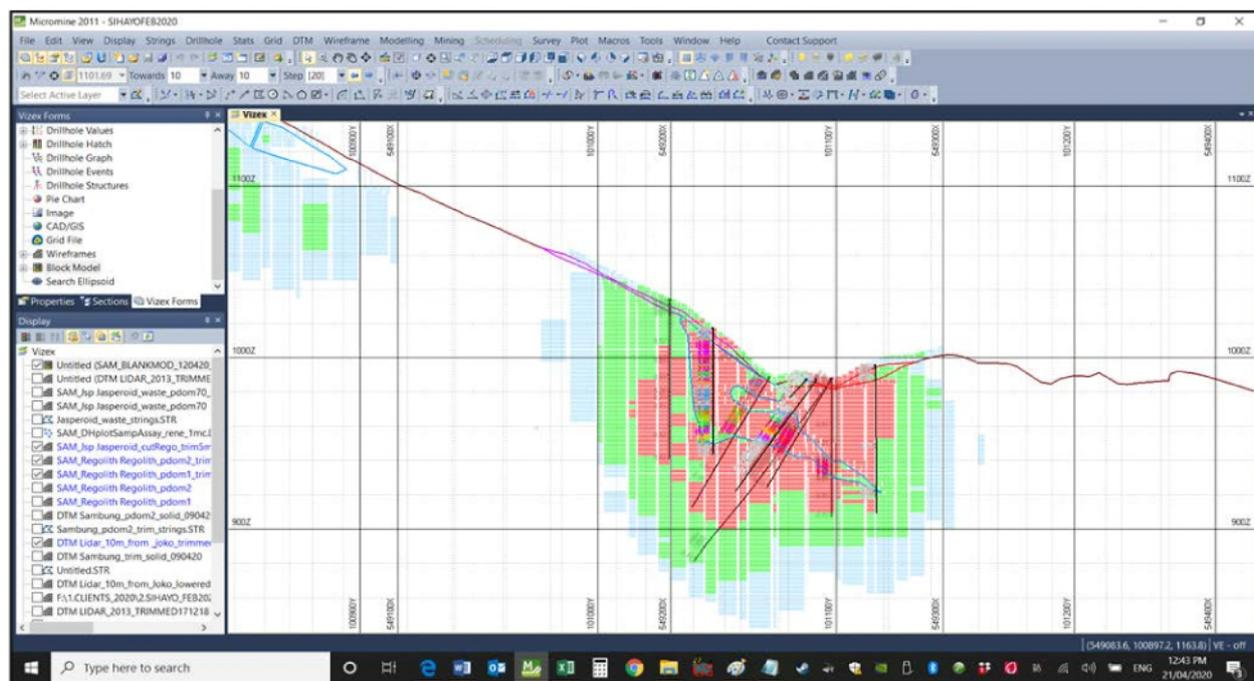
Figure 4-3. Figure 66: Sambung Sectional oblique view 3 of the block model displaying block resource categorisation
