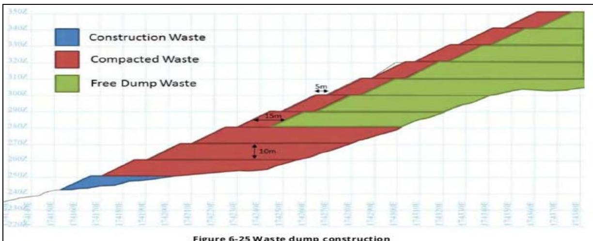
Figure 6-25 Waste dump construction
