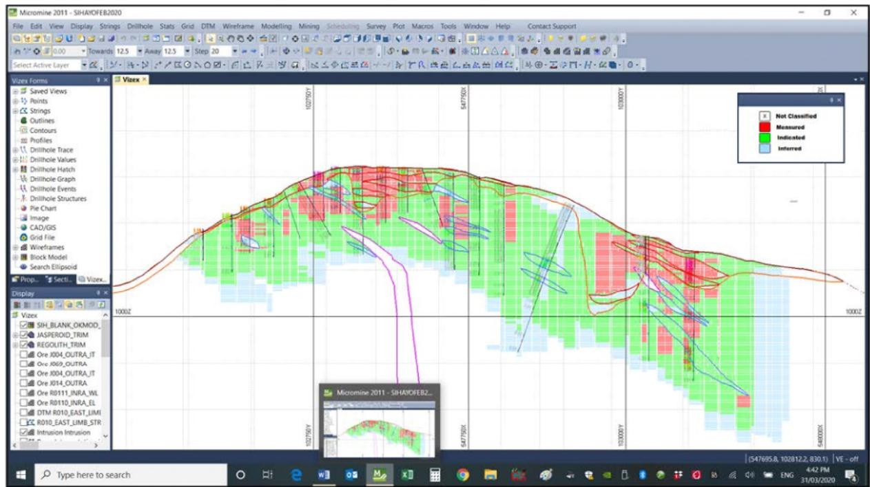
Figure 4-2. Sihayo Sectional view 54500mE of the block model displaying block resource categorisation (Figure 61).
