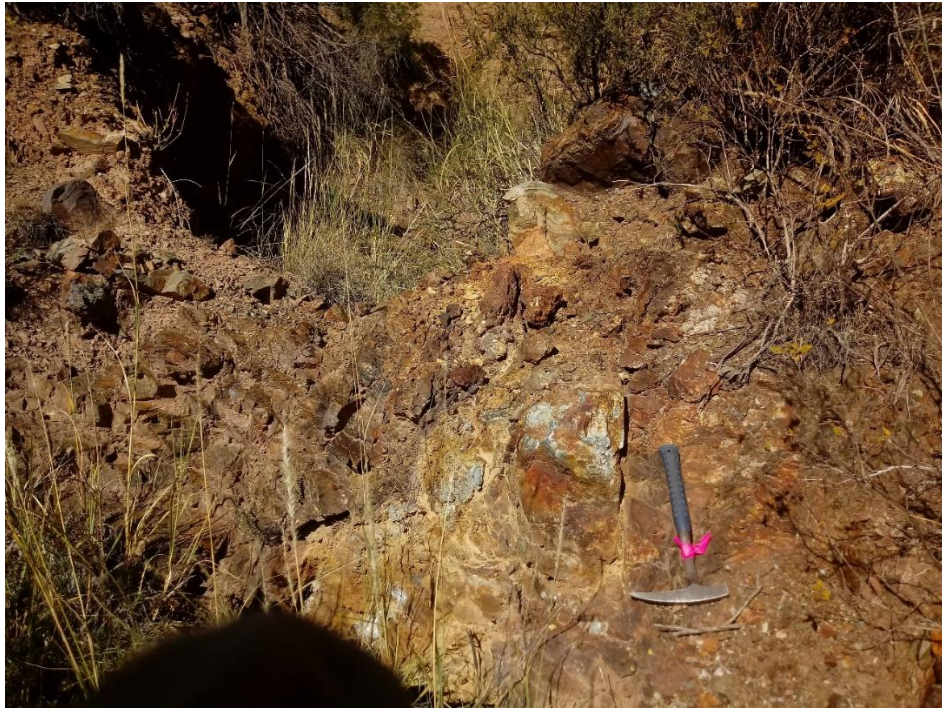
Figure 5: Mineralized quartz vein with sulphides and altered host rock - King Tut Mine (Source: Condor Prospecting Pty Ltd)
