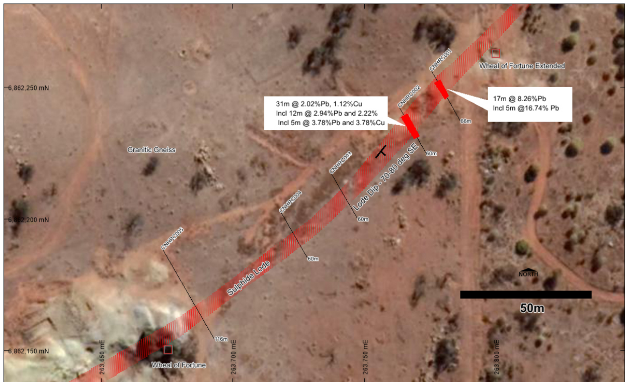
Figure 11: Plan view of Northampton drilling locations and results
