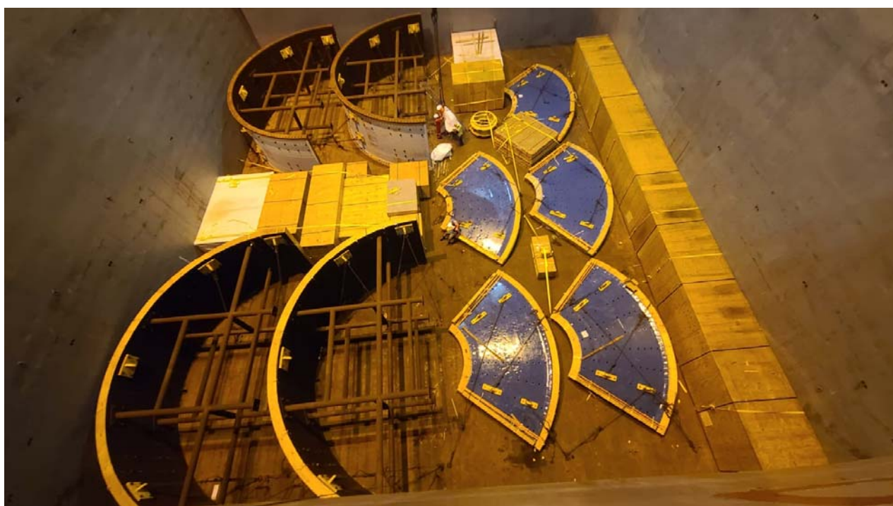
Figure 2: Part shells of the 36-foot SAG mill loaded for transport.
