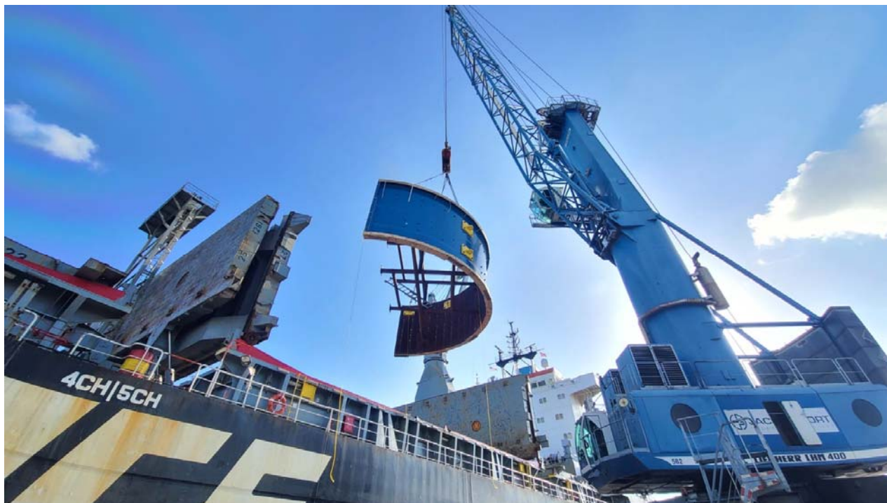
Figure 1: Part shells of the 36-foot SAG mill being loaded for transport.
