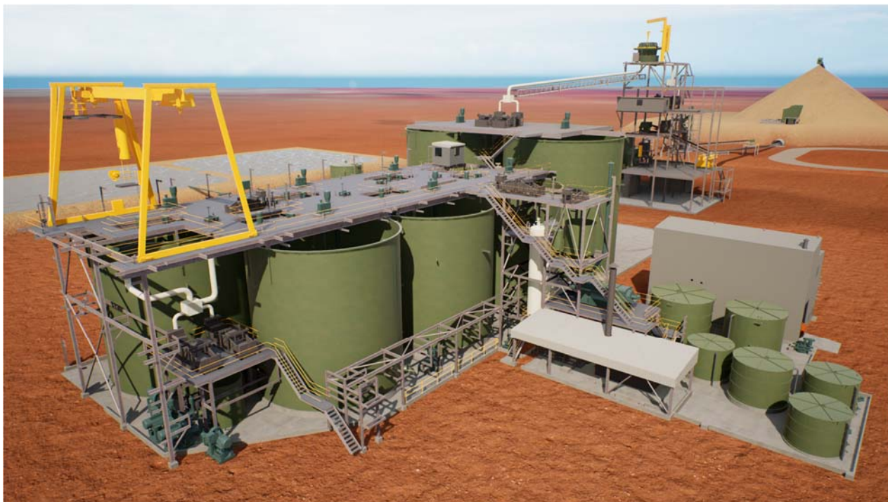
Figure 3: Artist's impression of the planned 4Mtpa CIL plant at King of the Hills.
