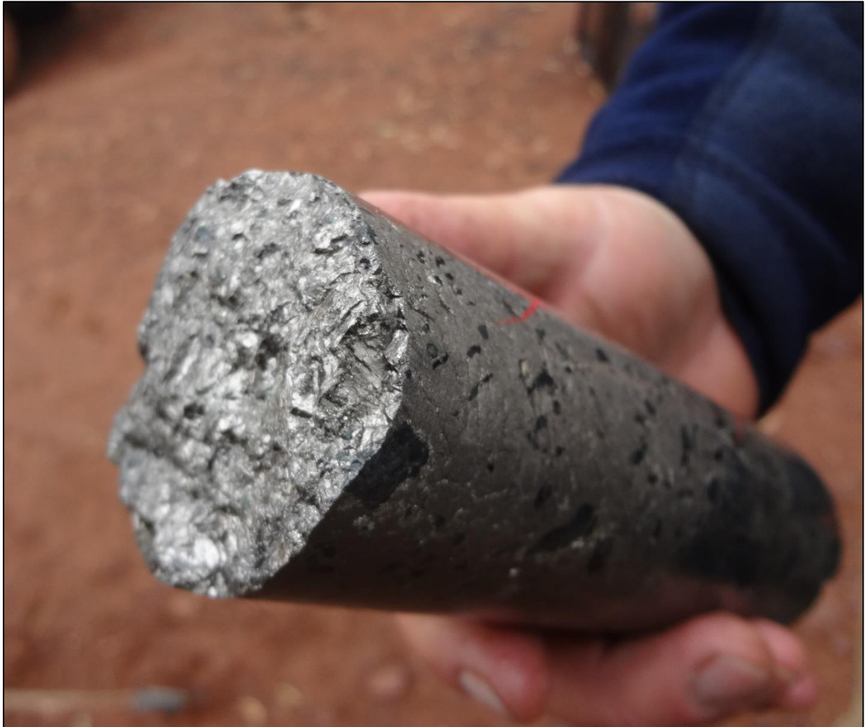
Figure 2. Ni-Cu bearing massive sulphide zone in diamond drill hole CBDD030 drilled 300m south of the T5 Ni-Cu discovery zone (438.3m-438.5 shown).
