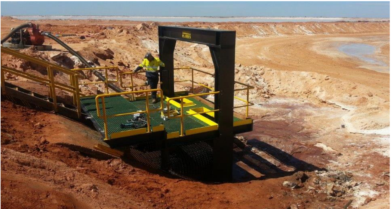
Figure 7.3. Typical Weir Platform Installation for Ponds
