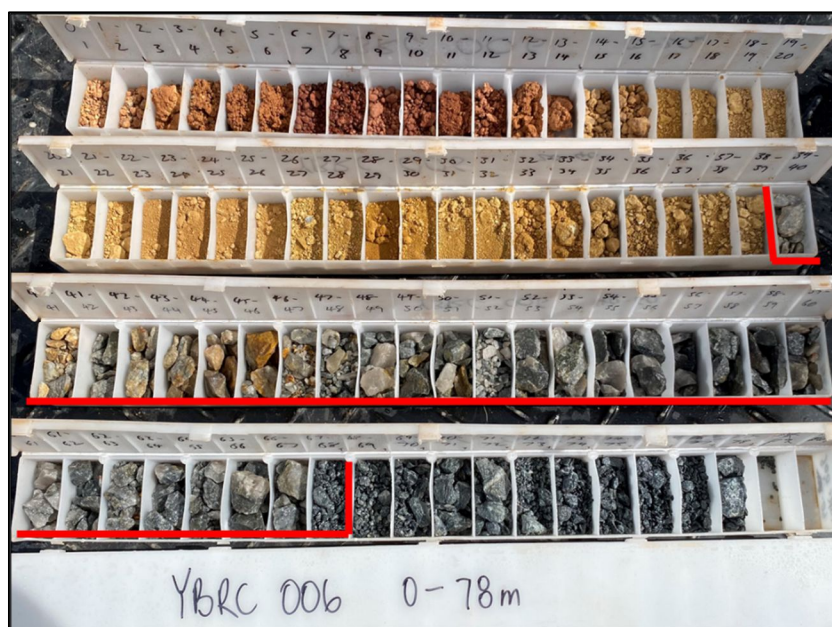
Figure 3 YBRC006 chip tray showing 29m intersection of massive veining, porphyry with iron sulphides
