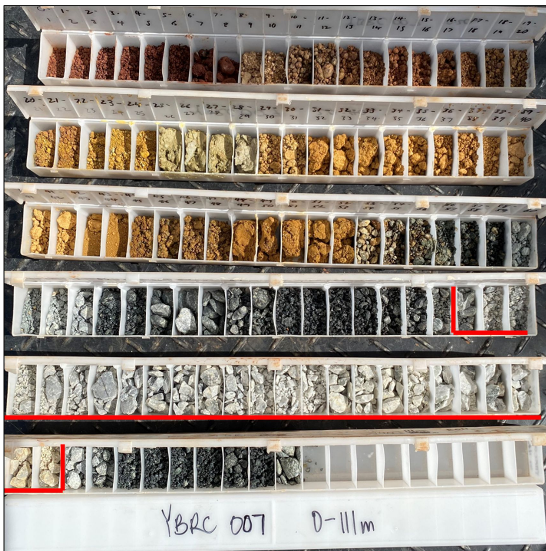
Figure 4 YBRC007 chip tray showing 25m intersection of massive veining, porphyry with iron sulphides
