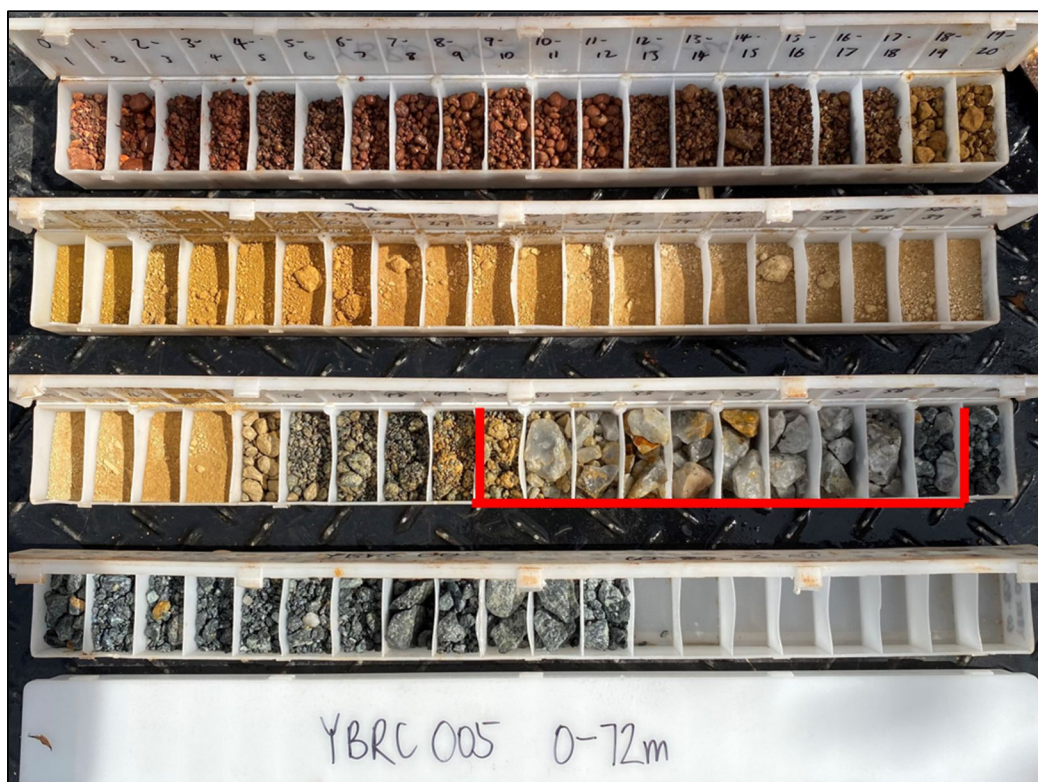
Figure 2 YBRC005 chip tray showing 10m of massive veining with minor sulphide mineralisation
