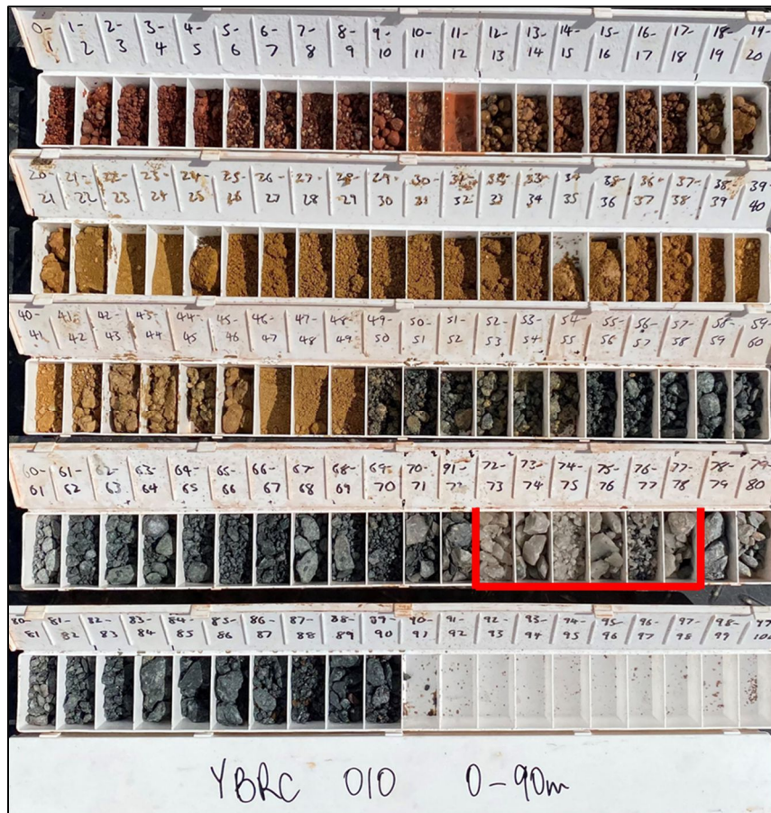
Figure 7 YBRC010 chips showing 35m of weathered veining, clays, quartz-feldspar porphyry with sulphide mineralisation
