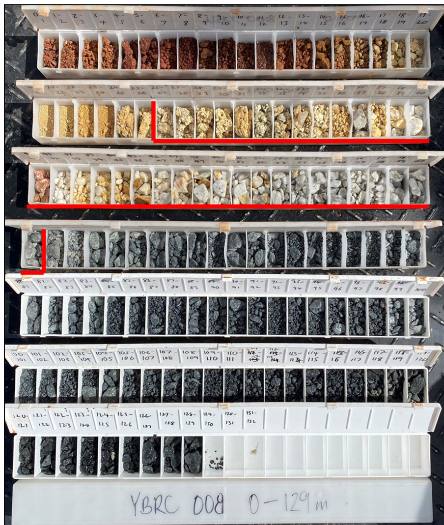
Figure 5 YBRC008 chips showing 35m of weathered veining, clays, quartz-feldspar porphyry with sulphide mineralisation
